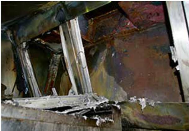
Figure 8: Burnt grease filters.
